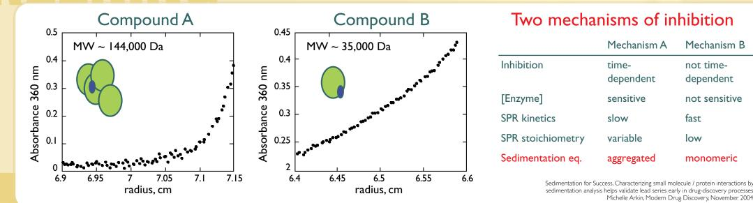
Two compound series shown to result in a relative change in the sedimentation profile of the molecular weight complex. The aggregate species is clearly shown to produce an exponential-like profile.
