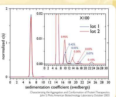
Comparability of conformation and aggregation for two different manufacturing lots of a monoclonal antibody with results from both lots showing good homogeneity (98.6% main peak or better) and the same molecular conformation based on reproducible sedimentation coefficients (6.339 S for lot 1 and 6.335 S for lot 2).
